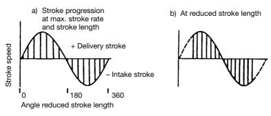
Set stroke length dependent on the required delivery capacity.
